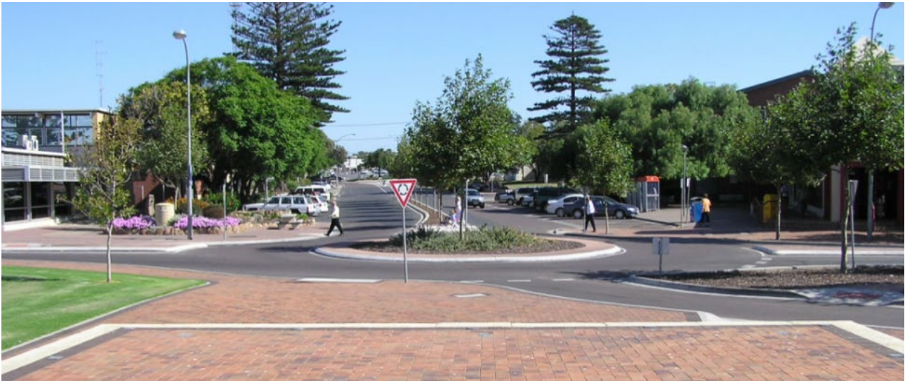
Figure 7.3: Example of a landscape treatment at a roundabout within a shopping precinct
