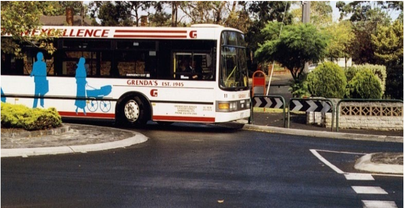
Figure 4.9: Front overhang on low-floor bus
