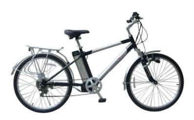
The maximum power assistance is 200 watts and the power should cut out when the bike reaches 25 kilometres per hour. Cyclists must be 16 years old or over to ride an electric bike, and do not need any form of driver's licence.
